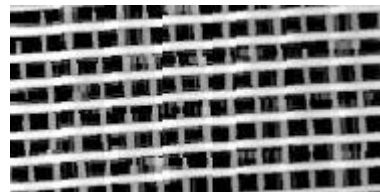
Accurate mapping out of reinforcement
